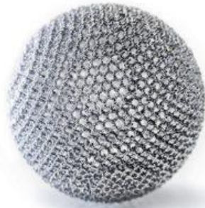
Figure 3 STRUCTURE OF TRABECULAR TITANIUM
